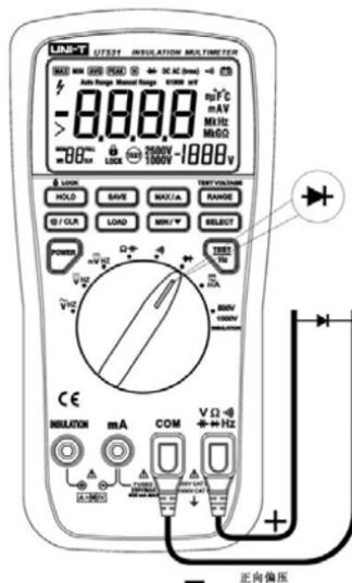
Figure 11. Testing Diodes
