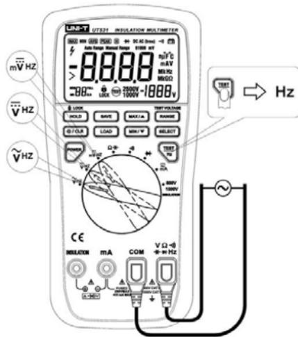
Figure 13.Measuring Frequency
