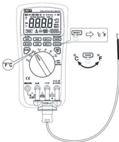
Figure 14.Measuring Temperature
