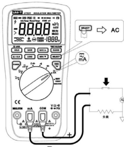
Figure 12.Measuring AC or DC Current
