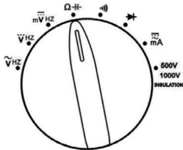
Figure 2. Rotary Switch
