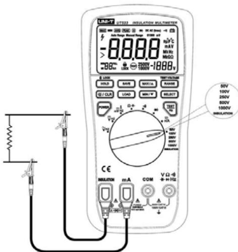
Figure 15. Testing Insulation
