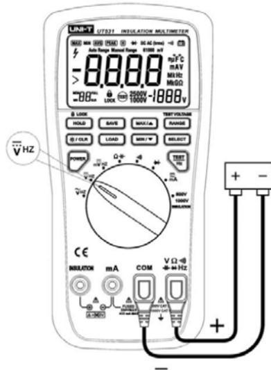
Figure 6.Measuring DC Voltage
