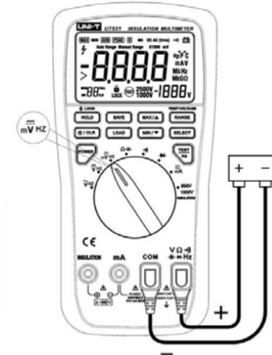
Figure 7.Measuring DC Millivolts
