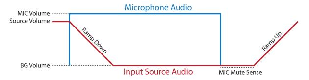
When using the microphone mixing functionality, it is recommended to only use 2ch audio sources, or set the EDID of the product to a 2ch EDID. While the MFP62 does support multichannel audio, mixing the microphone input over the multichannel signal is not possible hence the source audio drops out when the microphone audio is triggered. To enable multichannel audio support, you must choose a multichannel EDID via the Web GUI of the product.
