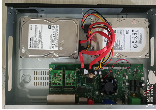
Figure 1-7 Connecting the Cable
