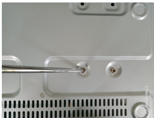
Figure 1-6 Fasten the hard disk
