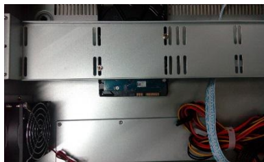
Figure 1-2 fasten the hard disk
