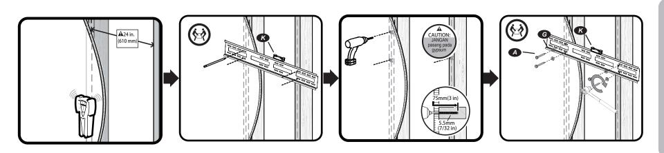
Attach mount to wall (Wood Stud wall)
