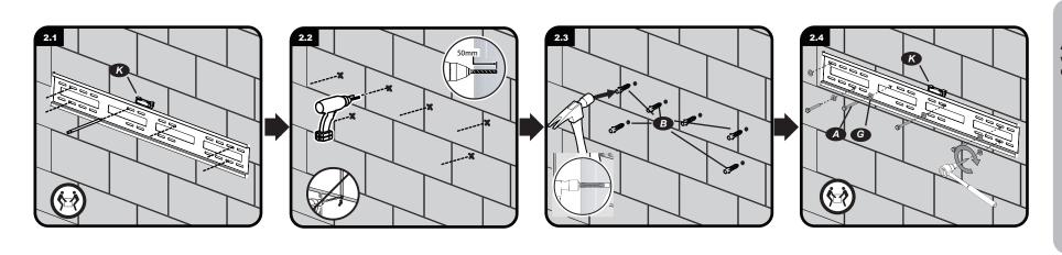
Attach mount to wall (Solid Concrete wall)
