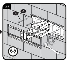
2 Attach mount to wall (Solid Concrete wall)
