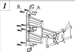
Using the bubble level to ensure the wall plate is level, Pre-drill 8 holes with a 10mm bit to 50mm deep. Insert wall anchors into the holes, then using long bolts to mount the wall to studs.
