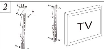
Using Long bolt(CorD), washer(F)and Spacer (E) to mount TV set to the aluminum siding.
