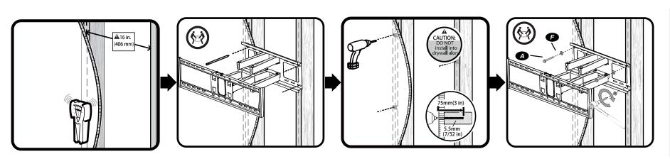
Attach mount to wall (Wood Stud wall)
