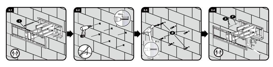
Attach mount to wall (Solid Concrete wall)
