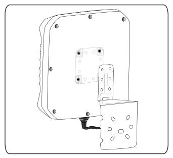
2.) Place the antenna back plate over the pole mounting bracket and attach using the 4 x M6 x 12mm bolts & washers.
