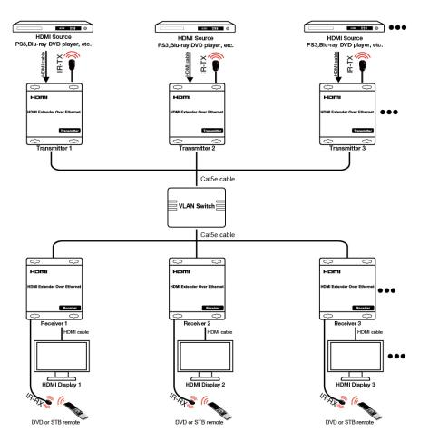
Some A HTTP server is embedded in TX and RX, you can setup IP address for RX via web browser. Please refer to "Setup HDMI TX and RX" in page 8.
