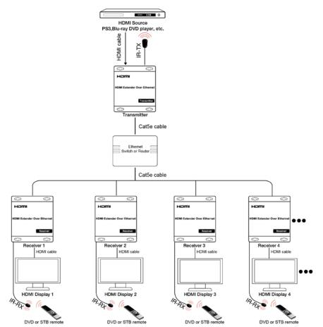
**Connect HDMI** Transmitter port and Receiver ports to the Ethernet Switch
