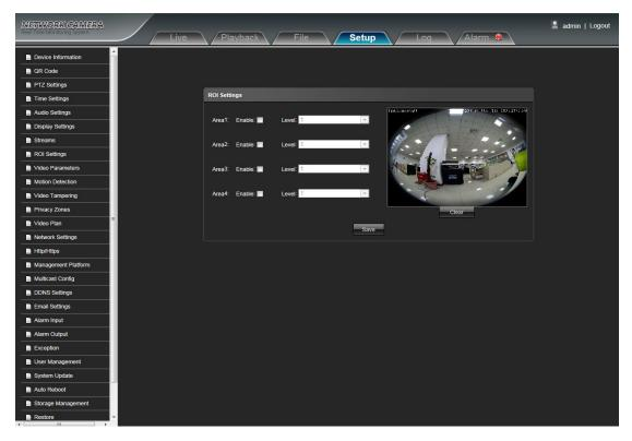
• **ROI Setting:** On the preview window, hold down the left mouse button and drag to set the ROI area. A total of four ROI areas can be set, click **Enable:** to set the corresponding ROI region coding level, the higher the level of coding, the stronger the ROI region encoding
