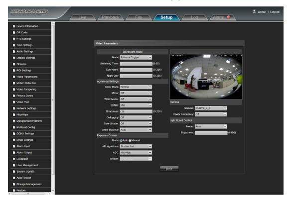
• Day&Night Mode: Outside Trigger/ Auto/ Color/ Black White four kinds of mode selectable. Non infrared IP cameras default mode is Auto, and infrared IP cameras default mode is Outside Trigger. According to the IP camera type and actual scene, user can select the Day&Night mode optional
