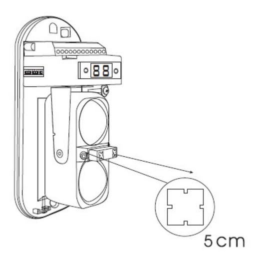
2. Vertical and horizontal adjust as below picture showed to get a best signal strength, if signal strength is less than 1.8, please adjust again to get a better signal strength.
