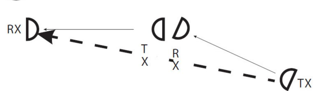
Multi sensors may be used for long-distance guarding. Please install according to the below diagram to avoic interference between beams.
