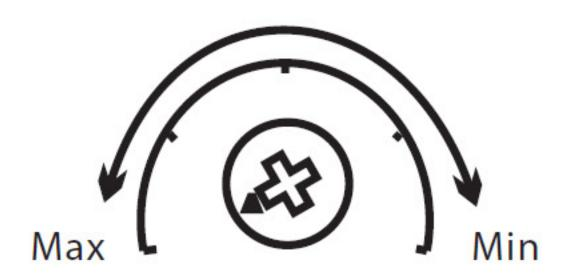
Please see the diagram to adjust the response time of the receiver. Usually, the time set shall be less than the time when the intruder corsses the grarding area. The MIN point is the shortest time. Time: 50-240m sec without degree
