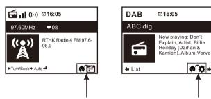
Press and hold the **< OK >** button, it will switch to the internet radio mode to play the corresponding channel.
