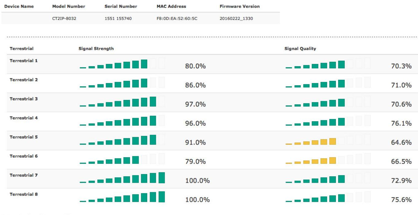
Overview Page will provide an overall system status of the CT2IP-8032 Converter state: Signal Strength and Signal Quality.
