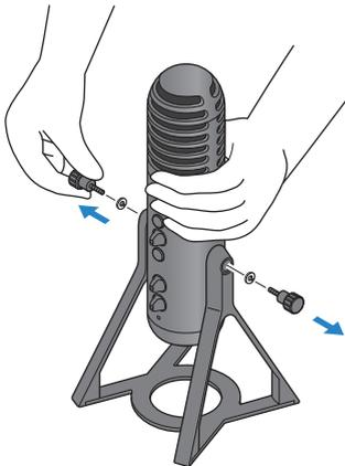
Attaching this product onto a mic stand or desk-mounted microphone boom arm > How to attach
