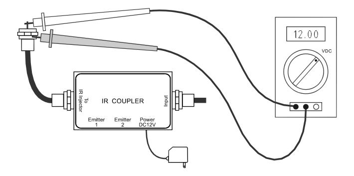
If you are troubleshooting a whole-house IR system and you measure approximately 8-12 Volts DC on the output of the IR COUPLER, but 0 Volts DC on the output of your RF splitter, check the following items:
