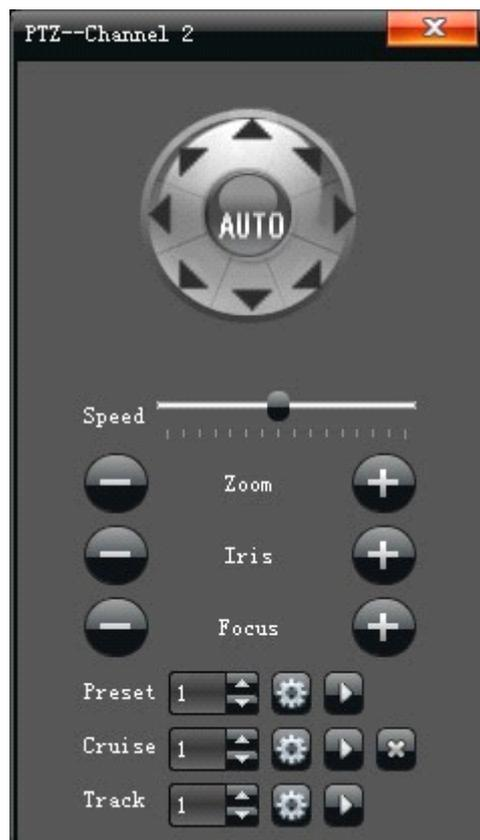
1) "Preset" setting: Rotate the camera to appropriate angle and position by PTZ directional buttons, select a preset number in the drop-down list, and click "⚙️" button.
