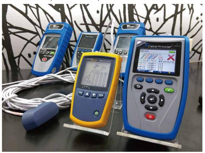
The color screen of the Cable Prowler shows its advantage again, and the length of each pair is displayed in this mode as well.
