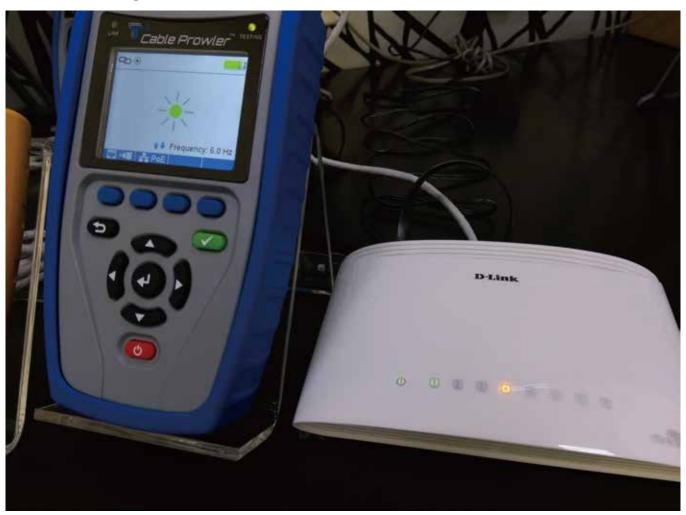
The Cable Prowler supports the link light function, by sending out a flash light signal, user could easily identify which port the cable is connected on the hub or Switch. Other features that come with the Cable Prowler only:
