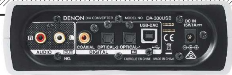
ABOVE: Self-evident sockets, so no need for the owner's manual: RCA phono line-out, one coax, one USB and two optical digital inputs, with DC power via a wall-wart
