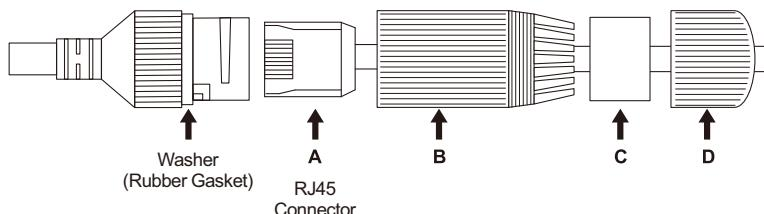
3. Install an RJ45 connector on the unterminated end of the Ethernet cable using an Ethernet cable installation tool.
