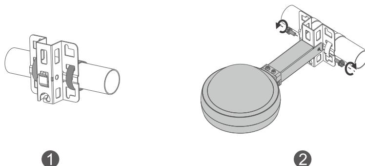
1. Secure the mounting plate to the horizontal pole by threading two clamps through the mounting plate.
