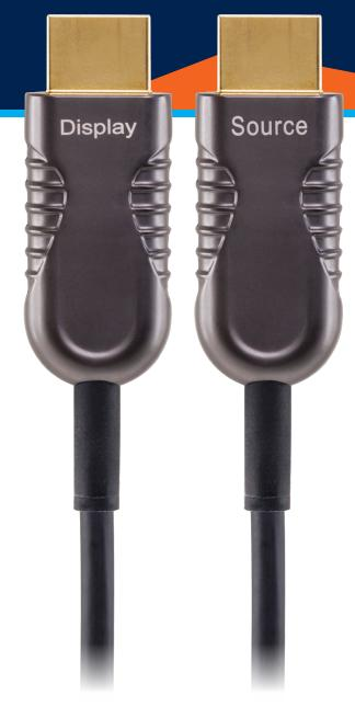
HDMI 2.0 Active Optical Cable (AOC) is used to extend the transmission distance between any HDMI sources and sink devices using a hybrid cable of optical fibres and copper wires. The high-speed TMDS signals are travel through the Optical multimode fibres, while the low frequency control signals are transmitted through the copper wires.
