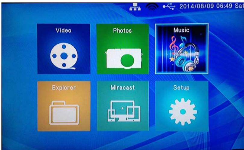
Using the media player's remote control, navigate to "Music" and press ENTER to select it. This will enable the music filter and take you to the device list. Once in the device list, use the navigation buttons to select the device type the media is located in. Depending on the size of the hard drive and the number of files it contains, it may take a few moments to detect.
