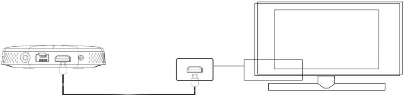
Connecting your media player to your TV via HD output provides the highest quality of visual output and high quality audio in a single cable. HD output can provide video resolutions of up to 1080p.
