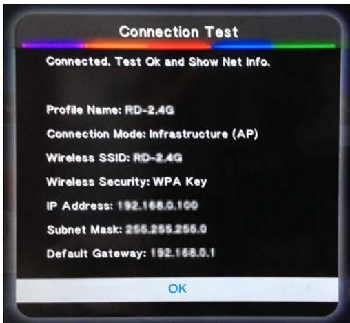
You can now access any devices that are connected to the Wi-Fi device by selecting network from any of the main menus.
