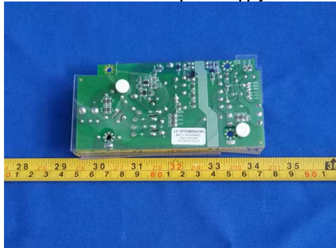
Photo 7 built-in power supply
