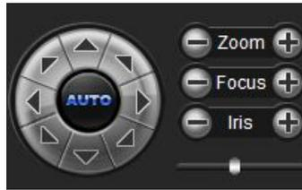
**PTZ Control:** You can use eight directional keys to rotate front-end devices, and AUTO indicates auto-rotation.
