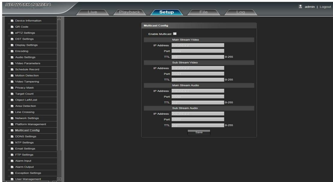
Multicast Config is in disable status by default. While click Enable Multicast, users can set the primary stream, sub stream, audio IP address, port, and TTL.
